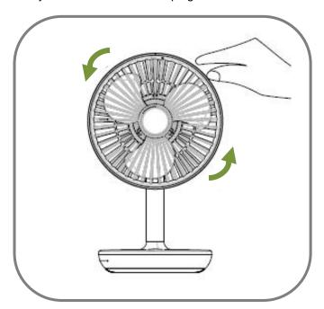
Remove the front of the fan by holding the back of the fan and turning the front guard anti-clockwise. Adjust the head of the fan, by pushing it backwards, to the maximum height.
