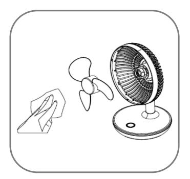
Clean the separate components of the fan using a soft dry cloth. Once clean reverse the process to put the fan back together.
