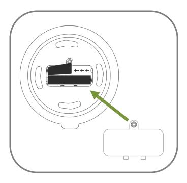
Insert new batteries (2 x 18650 3.7v 2500mAh lithium cell batteries), put the lid back in place and screw shut using a screwdriver.
