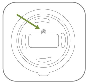
Turn the fan upside down and use a screwdriver to unscrew the lid on the base of the fan.
