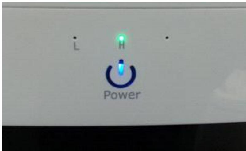
**Power** Press once to turn the humidifier on. Press again to toggle between low humidification and high humidification output.
